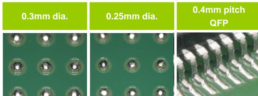
Larger relative surface areas of solder paste exposed due to miniaturization of components , often cause incomplete melting due to excess oxidation during the reflow. An improved flux formula ensures complete coalescence by minimum deterioration of barrier performances .
